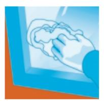
Degreasing the mesh: The mesh must be conditioned to degrease it and provide a key for the stencil. The type of conditioner used here is rubbed on with a cloth and heat dried.
