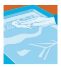
3. Place the stencil on a flat worktop and position the screen over it, printing side down. Dab the mesh with clean damp cotton wool until the stencil adheres completely to the underside of the screen.
