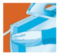
Cut the mesh to size, allowing an approximate 3cm overlap on each side of the frame. When attaching the fabric, staple through a thin strip of card to avoid tearing the mesh.
