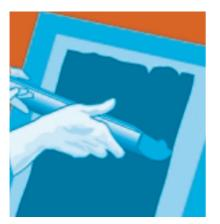
1. Fill a coating trough with light-sensitive emulsion. Draw the trough up the screen at an angle to lay an even coating of emulsion on the mesh.
