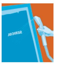
4. After exposure, wash the screen out with water. The emulsion has been hardened by the light but those areas protected by the positive image are washed away.
