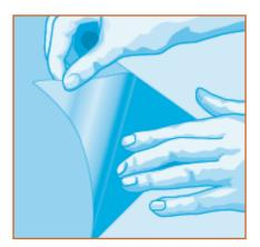
4. Dry the screen thoroughly and then peel away the transparent backing film, leaving the stencil on the screen mesh.
