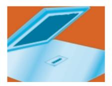
3. Position the light-sensitive screen over the positive. Close the exposure unit and expose the screen to ultraviolet light for the right length of time.
