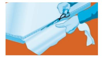
Use scissors or a sharp knife to trim off any surplus mesh around the edges of the frame.
