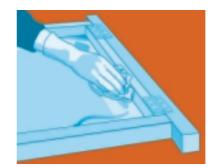
3. Wipe out the inside of screen and mesh with thinners and clean wipers. Rest the screen on sheets of newsprint and work until the mesh is quite clear of ink.
